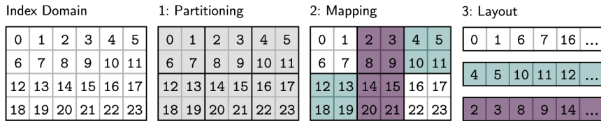
Figure 2.4: Example of partitioning, mapping, and layout in the distribution of a dense, two-dimensional array [FF16b]
